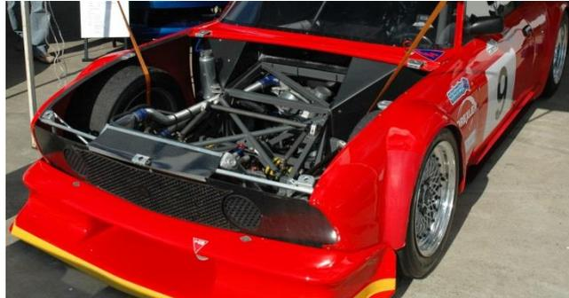
Suspension technology has progressed over the years to a point where the modern, higher budget Sports Sedan handles more like an open-wheeler due to them utilising a double wishbone coil-over front suspension or a rocker arm system. Rear suspension depends once again on budget; most front running cars use an independent rear suspension setup. Some competitors use a live rear axle setup with a watts-linkage/coil-over rear suspension.
